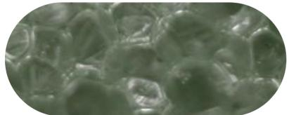
Polyisocyanurate PIR foam is very popular due to its high resistance to fire. Its defining feature in this regard is its ability to charr during combustion or when it is exposed to flame, due its "porous" carbon matrix. This matrix protects the inner layers and prevents them from burning. In addition, due to the structure of the matrix, significantly less heat is generated than with other foams which burn completely. The operating temperature of PIR Plita<sup>®</sup> is up to 120 °C.
