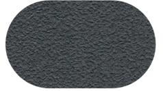
Fiberglass base with additional graphite and flame retardant coating. For use on the external cladding of walls and facades. Density  $630-700 \text{ g/m}^2$ , thickness 1.10 mm (± 15%)
