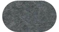
Bitumen coated fiberglass base with polypropylene. Mainly used on the construction of pitched roofs and flat roofs. Density  $330-370 \text{ g/m}^2$ , thickness  $0.72 \text{ mm} (\pm 15\%)$
