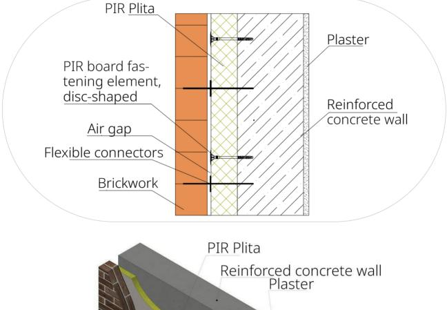
Disc-shaped dowel Brickwork Flexible connectors Air gap
