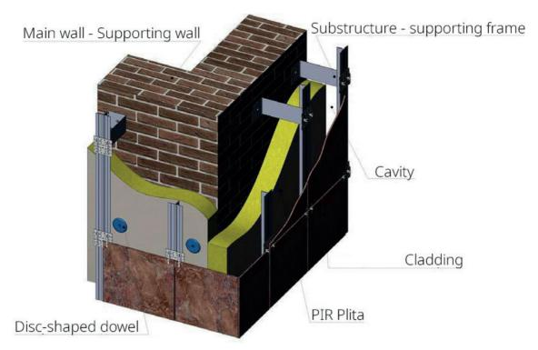
The attaching of PIR Plita<sup>®</sup> to the wall should be done using disc dowels. The insulation boarding is fixed to the brackets and then mounted. After that, the cladding is attached.
