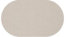
Fibreglass base reinforced with fiberglass mesh and mineral coating. For use on the external insulation of walls and facades using plaster. Density  $450-500 \text{ g/m}^2$ , thickness 0.7 mm (±15%)
